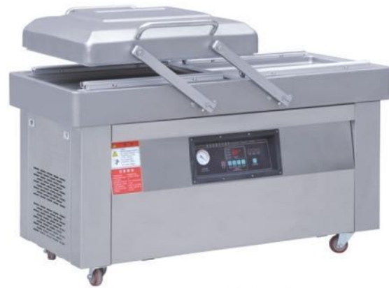
DZ-500/2SB 双室真空包装机 DOUBLE CHAMBERS VACUUM PACKAGING MACHINE
