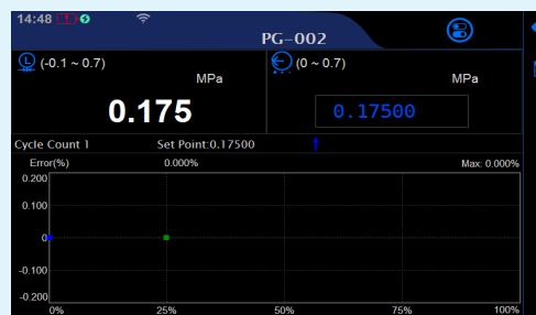
Pressure gauge / transmitter / switch calibration
