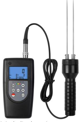
Soil moisture is important component of soil, which plays an important role in the growth of crops. The instrument measures the moisture content of soi.
