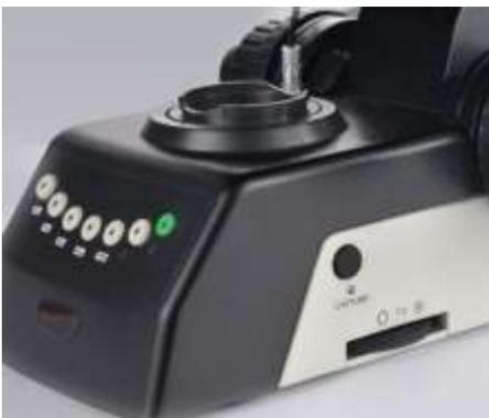
There is a cable from the microscope, the cable could be connected to the digital camera, after connection, just press the "CAPTURE" button at the right side of the microscope base, then you could capture the image easily.
