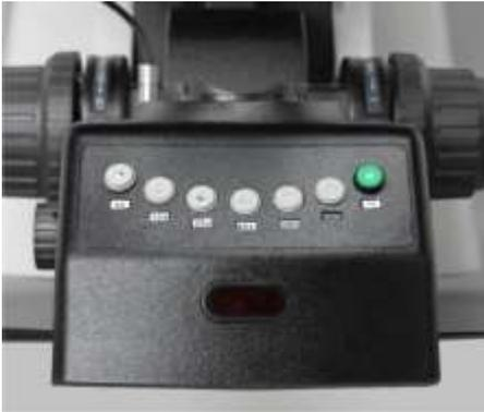
Objectives could be switched by simply pressing the buttons. Users could also self-define two of the most commonly used objectives and switch between them with the green button.
