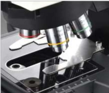
The top-lens on the condenser will be automatically swing-in or swing-out according to the objective lens that is selected.
