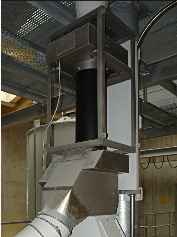
Installation example: Metal separator RAPID DUAL used for machinery protection during wood pellet production (old version)
