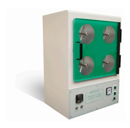
The RANDOM TUMBLE PILLING TESTER is used to determine the pilling and fuzzing characteristics of textile fabrics
