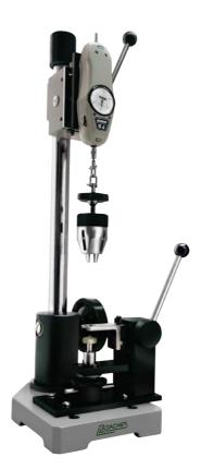
The OPTI-SNAP provides standard mechanism that increases test capability and repeatability. Our standard kits are designed for Next, GAP, H&M and Marks and Spencer test methods
