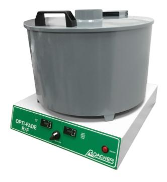
The OPTI-FADE is specifically designed to perform accelerated light fastness testing on textile samples in accordance to BS 1006
