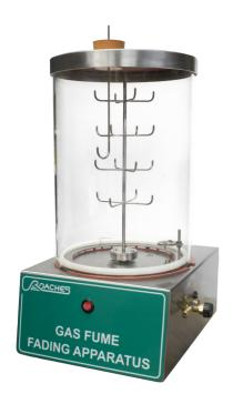
The GAS FUME FADER meets specifications required for establishing a specimen's colour fastness when exposed to atmospheric contaminants
