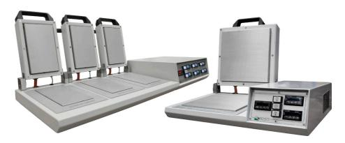
The CONTACT HEAT Test Unit has been developed to allow a wide range of tests to be carried out, where accurately controlled dry heat conditions are required on the surfaces of two flat heater plates.
