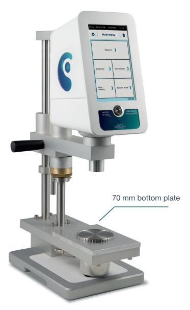
Equipped with a fluid circulation for temperature control (bath not included), the RM100 CP1000 PLUS will allow you to perform cone-plate and beaker measurements using the MS RV, MS VANE or MS KREBS mobiles.
