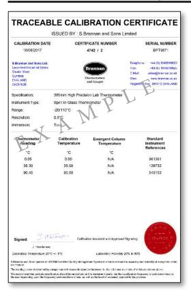
Following of the ban on specification mercury laboratory thermometers in October 2017, **Brannan** has developed a range of spirit filled, high precision thermometers. These thermometers are supplied complete with a traceable calibration certificate and are presented in a sturdy box for storage. The thermometers are made to the highest possible standards and are checked at every stage of manufacture to the requirements of our ISO 9001 quality management system.
