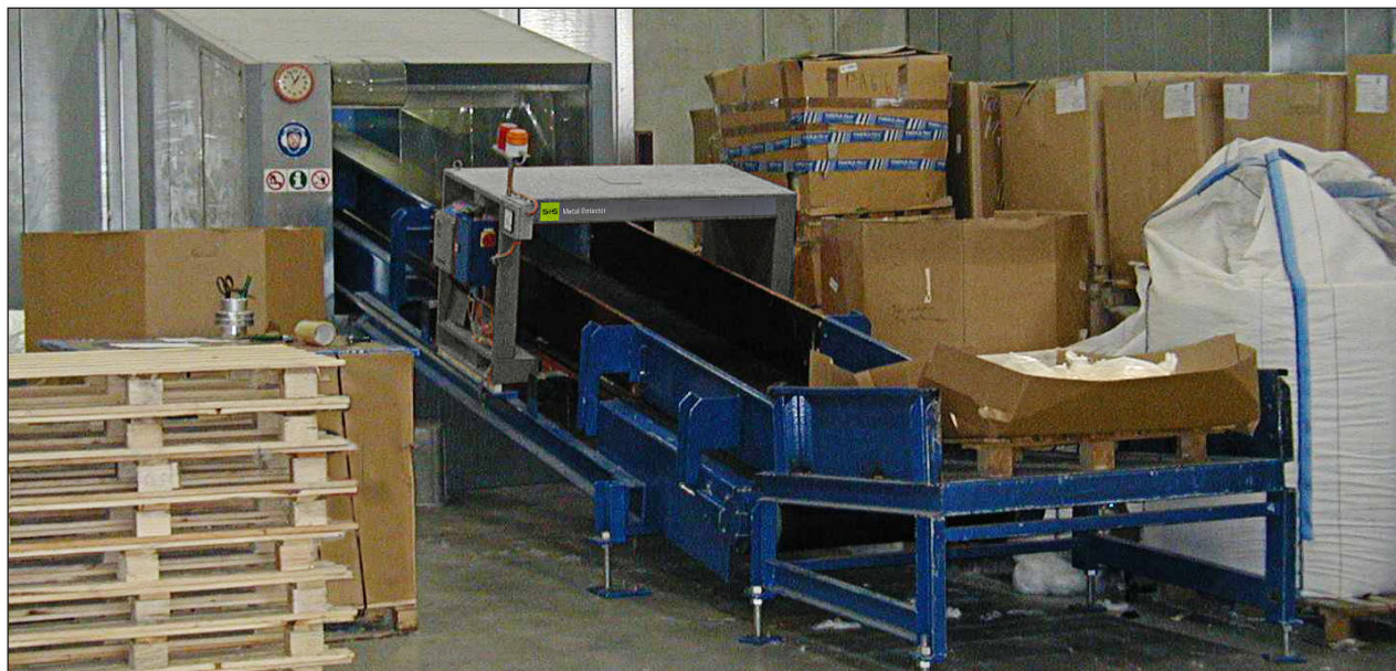
Installation example: Tunnel metal detector DLS analysing recycling material before the granulator. (old version)
