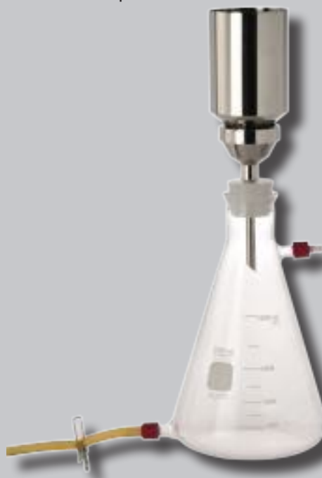
VF11 - silicone stopper Ø47mm, 500ml
