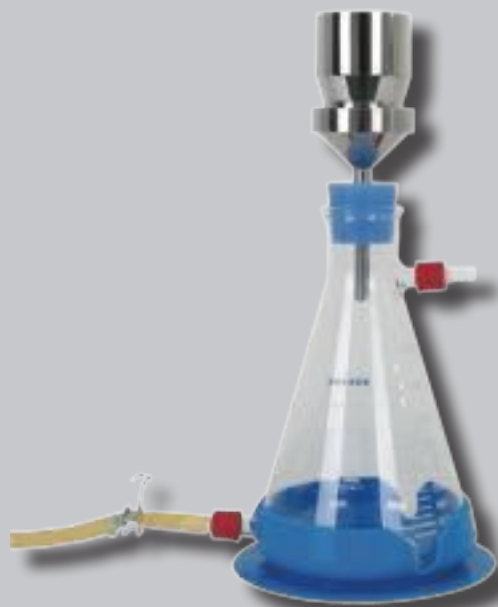
VF2 - silicone stopper Ø47mm, 100ml
